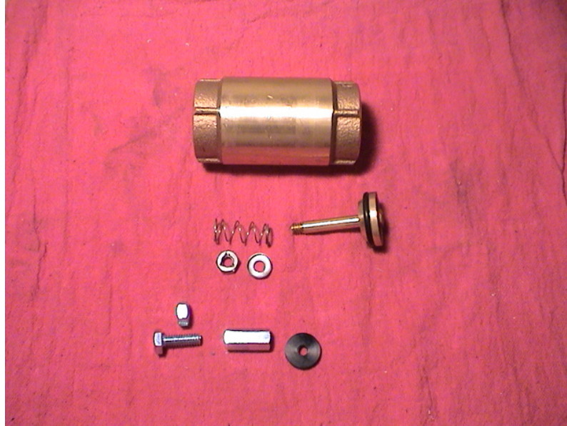
1" One way check valve disassembled.
