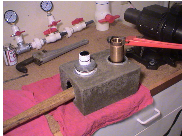
Installing the one way valve. Arrow up.
