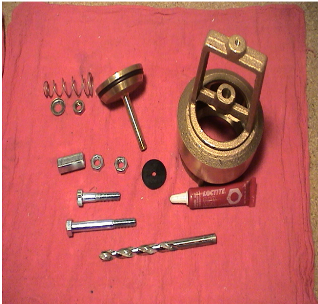
2" Foot Valve disassembled with parts
