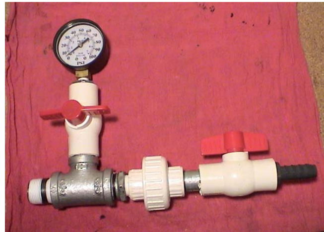
Completed Valve / Gauge Assembly
