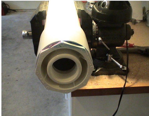
4" Slip x 2" FPT Bushing Glued in
