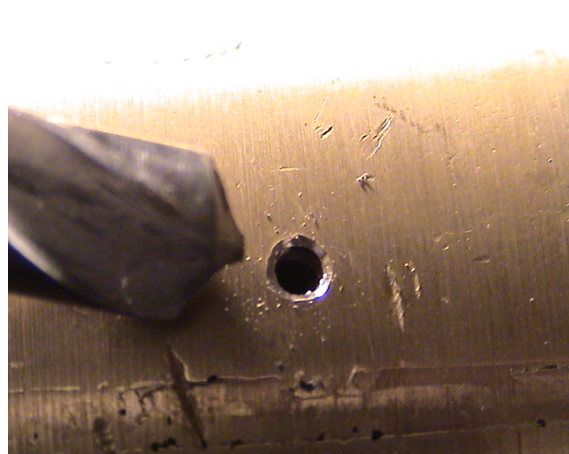
Adding a chamfer
