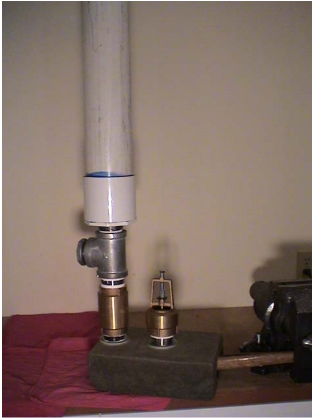
Pressure Chamber Installed
