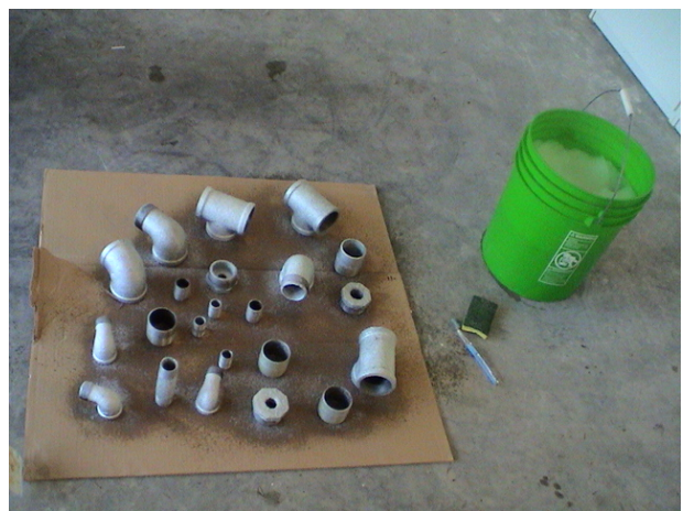
Galvanized parts with oven cleaner
