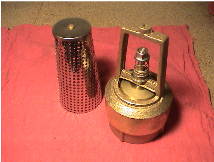
2" Brass Foot Valve with screen removed
