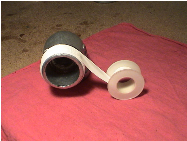
Wrap the Teflon tape clockwise
