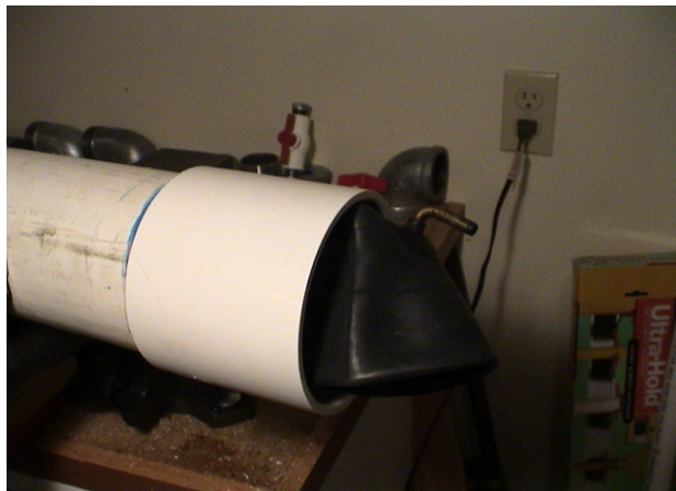
Inserting the inner tube with filler out
