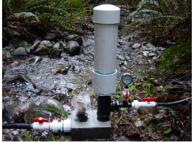
The 1" pump in action. 160psi poly drive pipe.
