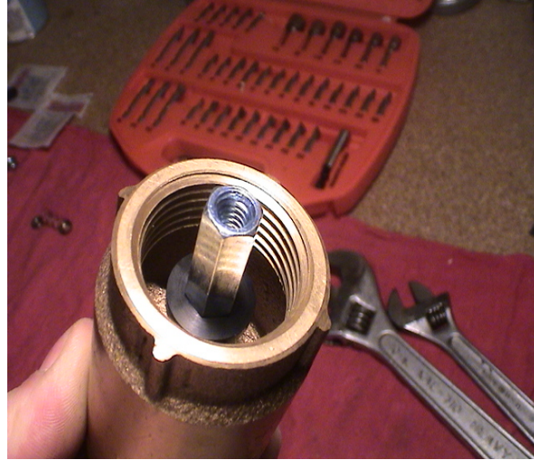
Faucet Washer and Coupling Nut installed.
