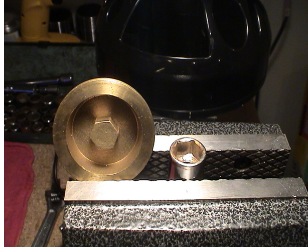
Clamping socket in vise to hold Valve
