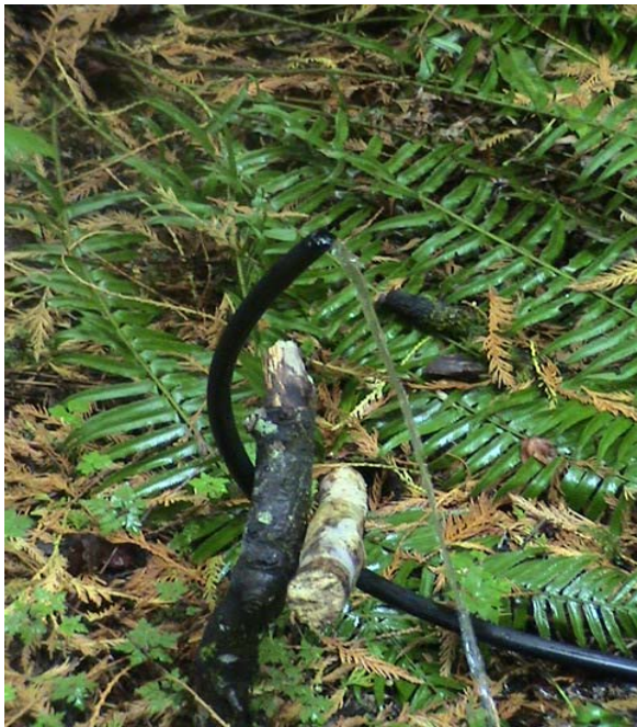
Delivery at top of ravine. 1gal in 37sec (2")
