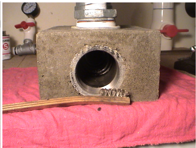
Cleaning the 2" threads with wire "toothbrush"
