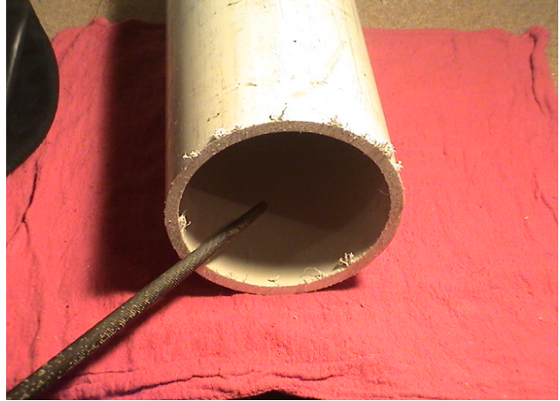
File off the sharp burrs and edges
