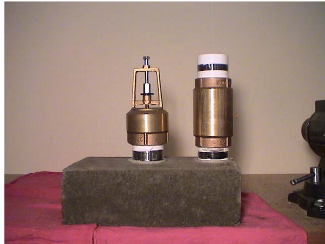
HRP2-2 Waste & Check Valve Installed
