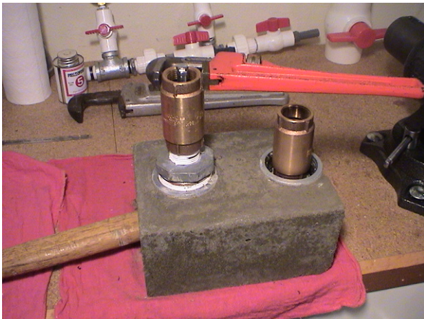
Attaching the Waste Valve
