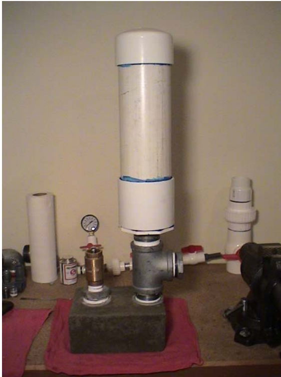
Pressure tank installed
