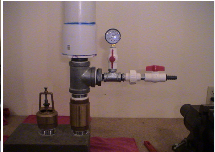
Adding the Pressure Gauge / Ball Valves
