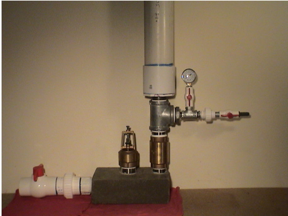
HRP2-2 Completed Pump, ready to paint
