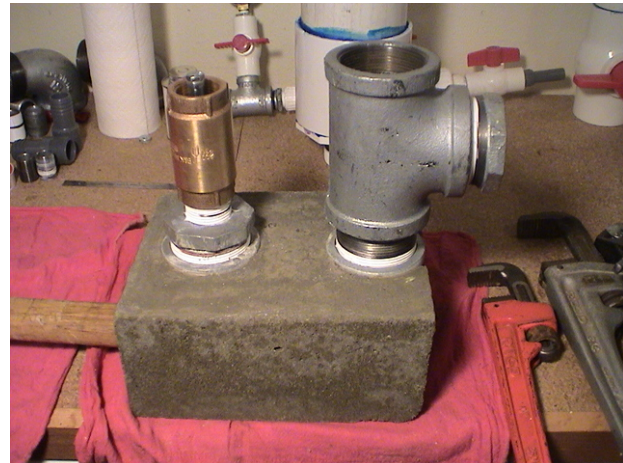
Attaching the "T" with bushing
