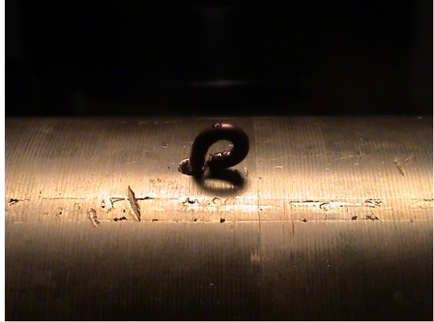
Wire through weep hole with twists
