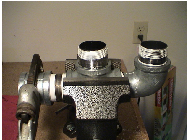
Adding the 2" Coupler after painting inside
