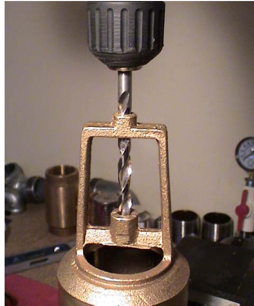
Drilling out to fit the 5/16" hardware
