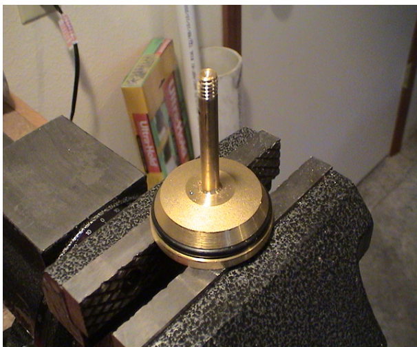
Valve stem held in socket
